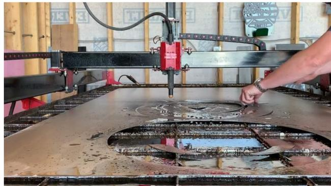
Gambar 2. 7 UnderWater Plasma Cutting (Stuff, 2021)
