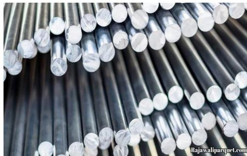
Gambar 2. 12 Aluminium magnesium silikon alloy
