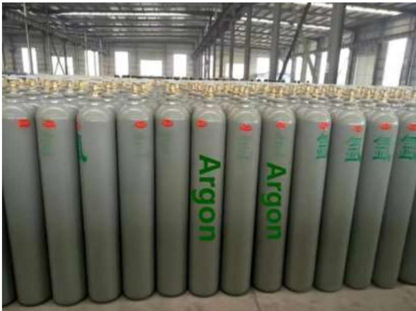
Gambar 2.10 Gas Pelindung (*Shielding Gas*)
