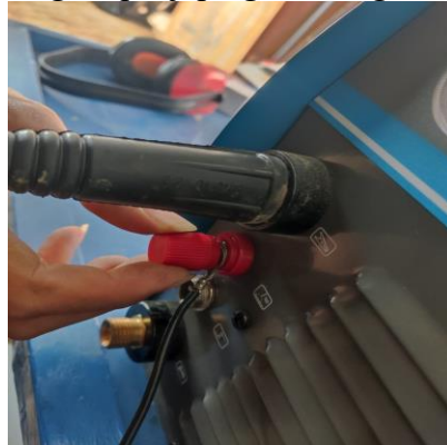
Gambar 3. 17 Penjepitan Kabel Grounding
