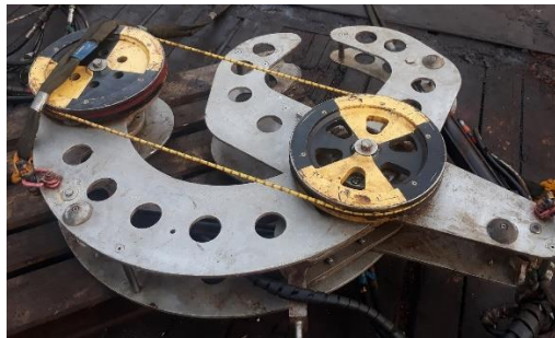
Gambar 2.1 Diamond Wire Saw (Worksprocess, 2024).
