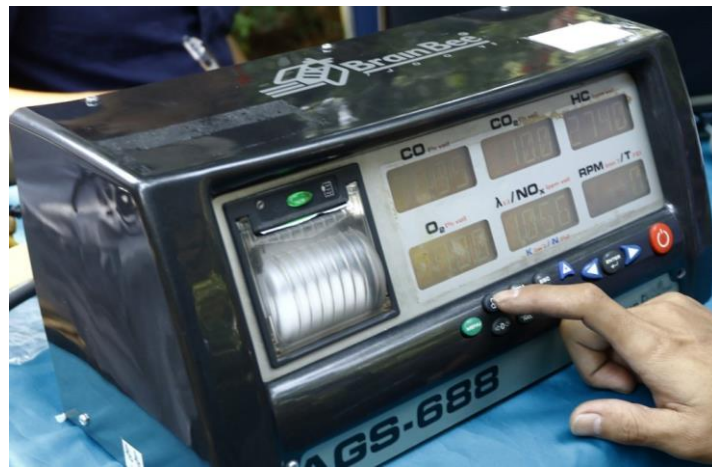
Gambar 2.8 Gas analyser (Tetuko, 2023)
