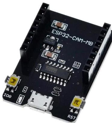
Gambar 2. 3 Modul Downloader Esp32 Cam
