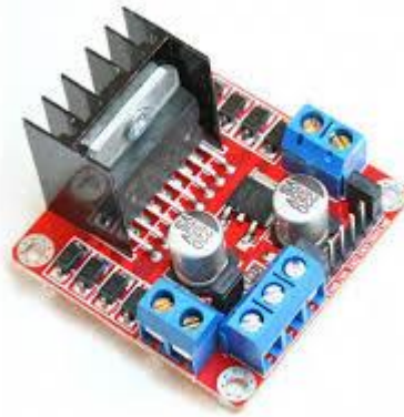
Gambar 2.14 Driver motor L298N
