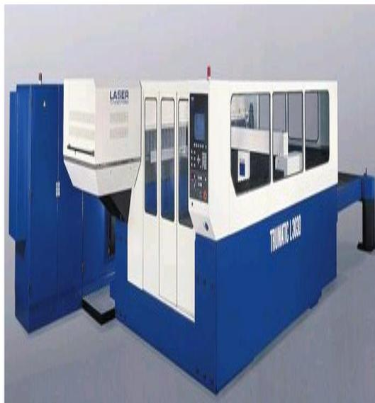
Gambar 2. 1 Laser *Cutting CO<sub>2</sub>* (Rakasita dkk., 2016)
