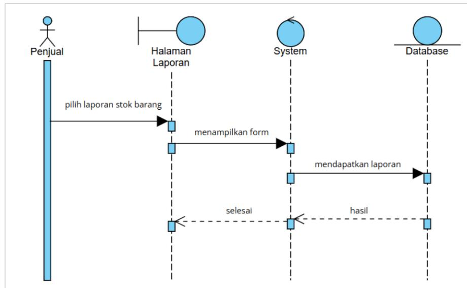
Gambar 4. 13 Sequence Diagram Laporan Stok Barang
