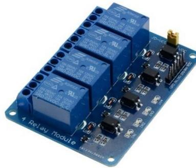
Gambar 2. 13 *Relay 4 Channel*
