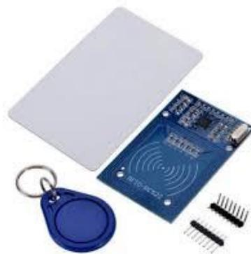
Gambar 2.5 *RFID(Radio Frequency Identification)*
