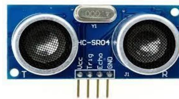
Gambar 2.4 Sensor Ultrasonik HC-SR04
