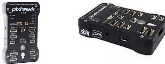
Gambar 2.7. *Flight Contoler Pixhawk*
