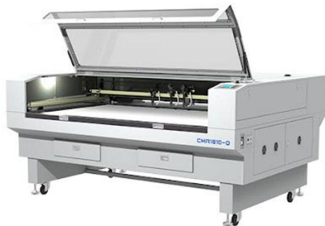
Gambar 2.2 CNC Laser *Cutting* CO<sub>2</sub>
