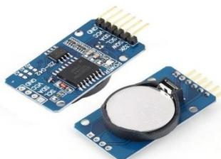
Gambar 2. 11 *RTC* (Real-Time Clock)
