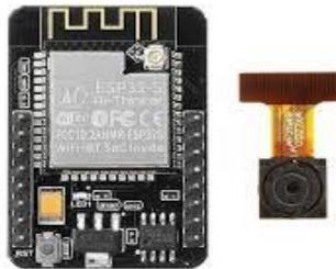
Gambar 2.2 *ESP32 Cam*
