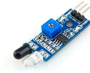
Gambar 2. 5. Sensor *Infrared*
