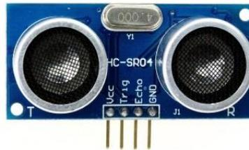
Gambar 2. 3 *Sensor Ultrasonik*
