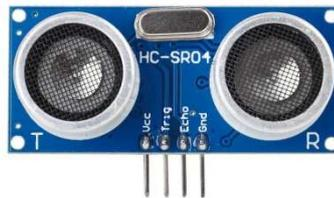
Gambar 2. 8 Sensor Ultrasonik
