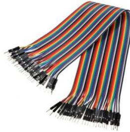
Gambar 2. 6 Kabel Jumper
