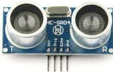
Gambar 2. 5 Sensor Ultrasonik HC SR04
