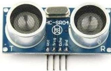
Gambar 2. 5 Sensor Ultrasonik HC SR04
