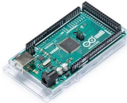
Gambar 2.1 *Arduino Mega*
