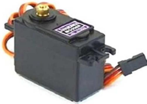
*Gambar 2. 5 Motor Servo MG996R*
