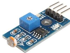
Gambar 2.4. *Module Sensor LDR*
