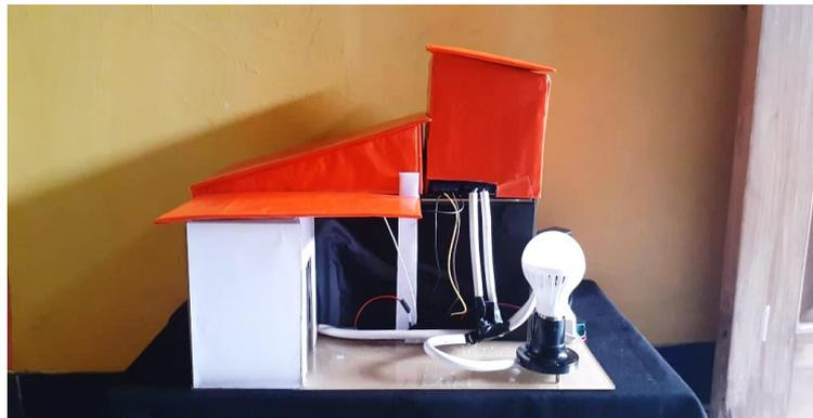
Gambar 5.1. *Prototype* alat Sistem Kendali Otomatis Rumah Pintar Berbasis Arduino
