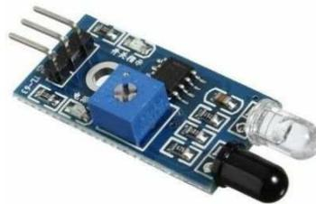
Gambar 2. 11 Sensor *Infrared*
