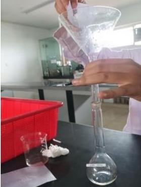
A person's hands are shown pouring a white powder from a glass funnel into a clear glass volumetric flask. The flask is held upright, and the powder is falling into it. In the background, there is a red storage bin and a laboratory bench. | Memasukkan Serbuk Kedalam<br>Labuu Ukur                 |
