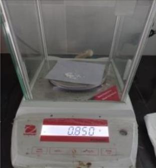
A digital scale with a white top and a red display panel. The display shows the number '0.850'. A small amount of white powder is visible on a weighing boat inside the scale's glass enclosure.                                                | Menimbang Serbuk $\text{AgNO}_3$<br>sebanyak 0,850 gram |
