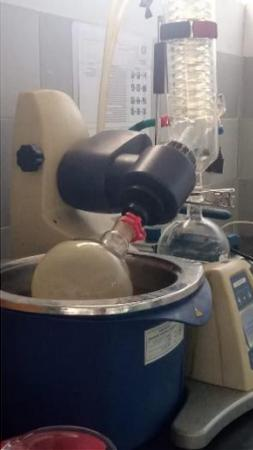
A rotary evaporator (rotary evaporator) setup, showing the main unit and a collection flask.                                                      | Proses rotary evaporator |
