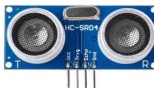
Gambar 2. 6. Sensor Ultrasonik
