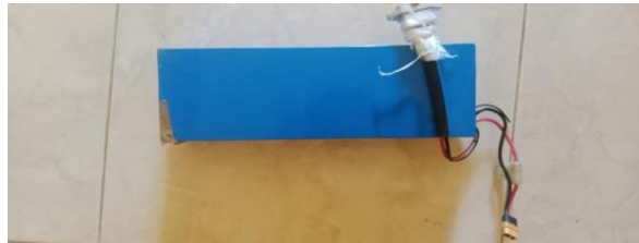
Gambar 3.5 Baterai Lithium-ion 48 V 10 Ah
