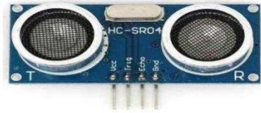
Gambar 2. 2 Sensor ultrasonik HC SR04.
