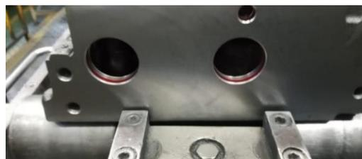
Gambar 4.8 Proses pembersihan lubang cylinder bore head
