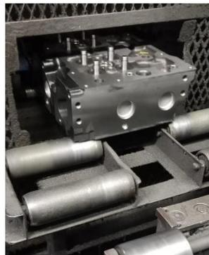
Gambar 4.7 Proses pembalikan cylinder head
