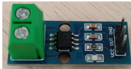
Gambar 2. 3 Sensor Arus ACS712
