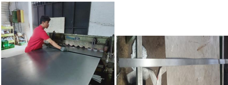
Gambar 4.6 Proses Shearing Plate Sheet SPCC
