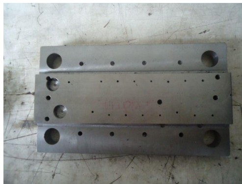
Gambar 2.28 Upper plate / Top plate (Allor P., 2023)
