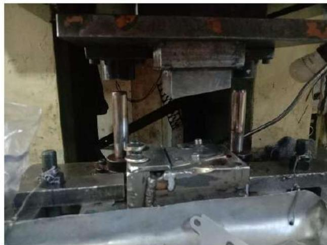
Gambar 3.5 *Bending dies*
