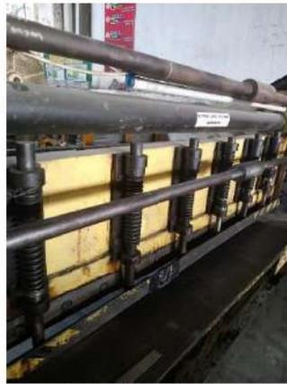
Gambar 2.7 *Tool holder driving*
