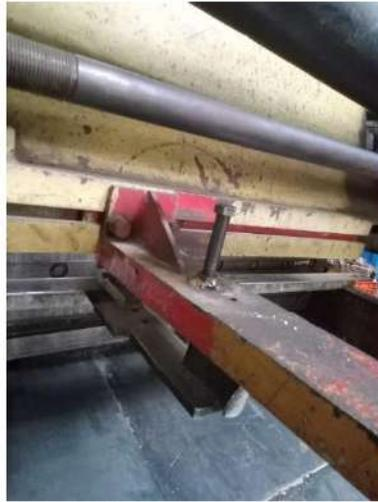
Gambar 2.11 *Rear Retaining Bracket*
