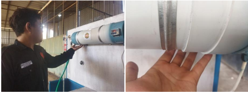
Gambar 4.27 Uji kebocoran Water Heater
