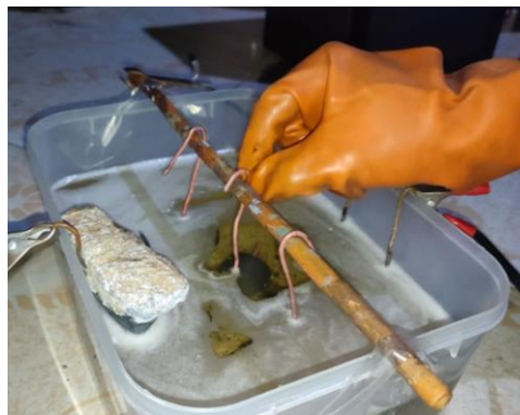
Gambar 4. 26 Eleketroplating waktu 4 menit
