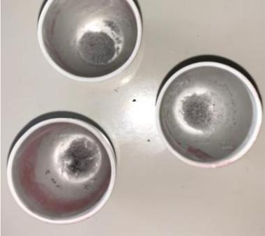
Three crucibles containing ash residue, likely from a gravimetric analysis.                                    | Uji Kadar Abu    |
