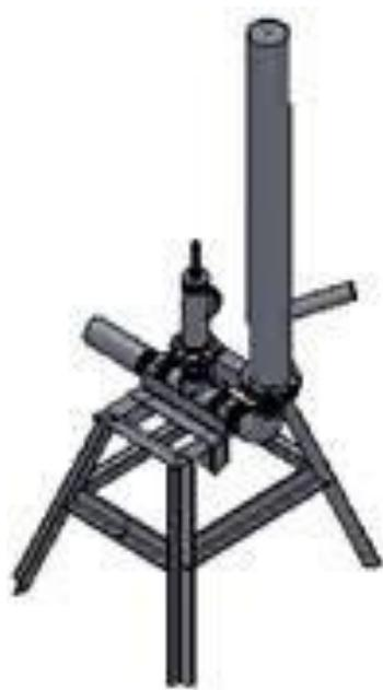
Gambar 2.3 Pompa Hidram
