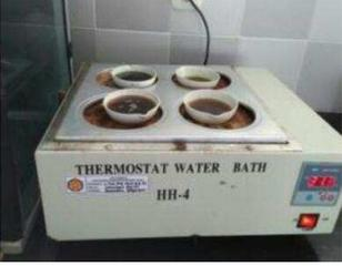
A white rectangular thermostat water bath with four small beakers placed on top. The front panel has the text "THERMOSTAT WATER BATH" and "HH-4". A digital display on the right shows "20.0". | Proses pengentalan ekstrak di waterbath |
