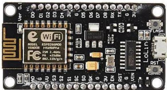
Gambar 2.5 NodeMCU ESP8266
