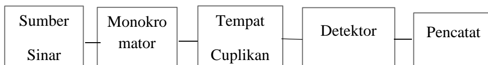
Gambar 2.5 Diagram Skematis Instrumen Spektrofotometer UV-Vis (Alfiyani, 2017).
