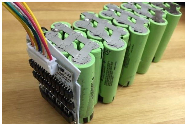
Gambar 4.7 Instalasi standar BMS
