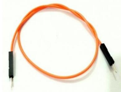
Gambar 2. 8 Kabel Jumper *Male to Male*
