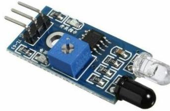
Gambar 2. 13 Sensor *InfraRed*
