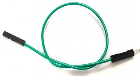
Gambar 2. 9 Kabel Jumper *Male to Female*
