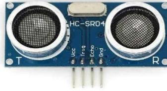
Gambar 2. 14 Sensor *Ultrasonik*
