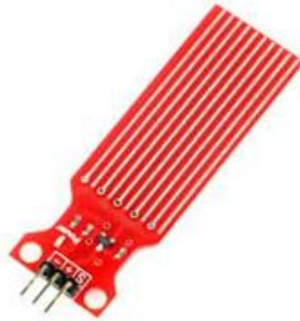
Gambar 2.1 *Water Level Sensor*
